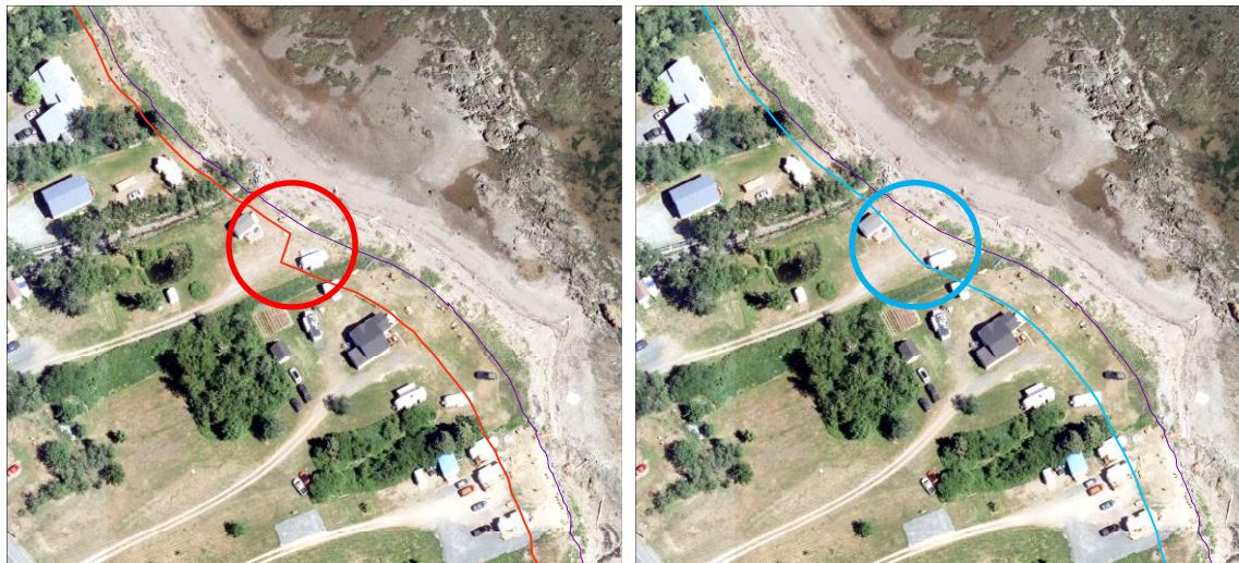
Figure 5. Erosion scenario for 2100 (a) without smoothing in the left side, (b) with smoothing at the connections between the homogeneously changing sectors in the right side.
