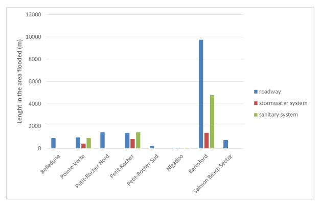
Figure 13: Length of roadway, stormwater system and sanitary system in the area flooded by a water level of 3.7 m. Only Pointe-Verte, Petit-Rocher, Nigadoo and Beresford have a stormwater and sanitary system. Nigadoo stormwater system coverage (GIS layer) is not available.
